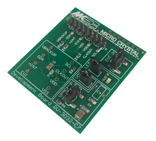
Temperature Compensated RTC Module
